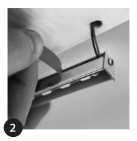
Remove backing from adhesive tape.
